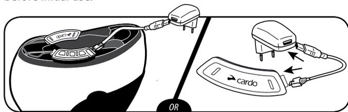
Charging with the wall charger is faster than via a computer USB port.
